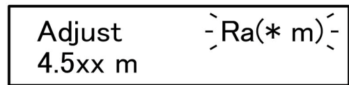
Figure 17: After Figure 16 process, you will see AEU name (in this example it is Radiator) start blinking again. If you want to adjust another element, use \text{\textcircled{0}} UP or DOWN to choose it.
