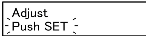
Figure 14: [Push SET] is blinking. Press \text{\textcircled{1}} SET to select what AEU to adjust. Figure 15 shows you selected [Ra].
