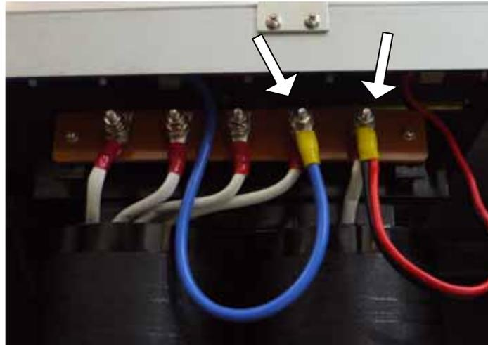
4. Make sure no wrong wiring or short circuit, and then put the left side panel to original position.
