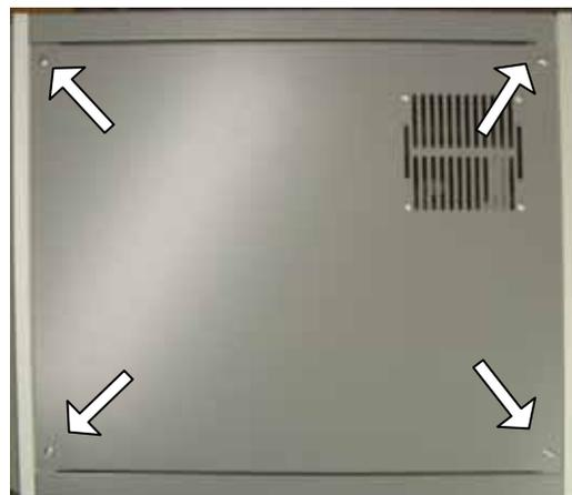
1. Removing nine screws to take off rear fan cover.
